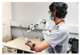
intuitive operation (Artemiadis, 2012) (Dwivedi, 2021). EMG-based systems can also allow for handfree interaction with robotic devices or computer applications. In this work, we propose development of data acquisition framework for real-time processing of EMG signals for the control of a robot armhand system.
